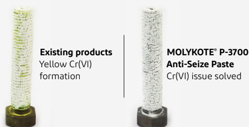
Lubricated stainless steel bolts after exposure to >500°C
