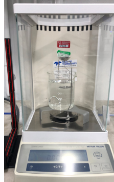
Figure 2. Balance fitted with a density determination kit
